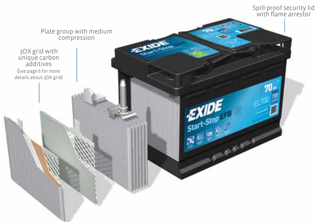
Positive plate: 3DX grid and advanced glass mat retainer covering active mass
